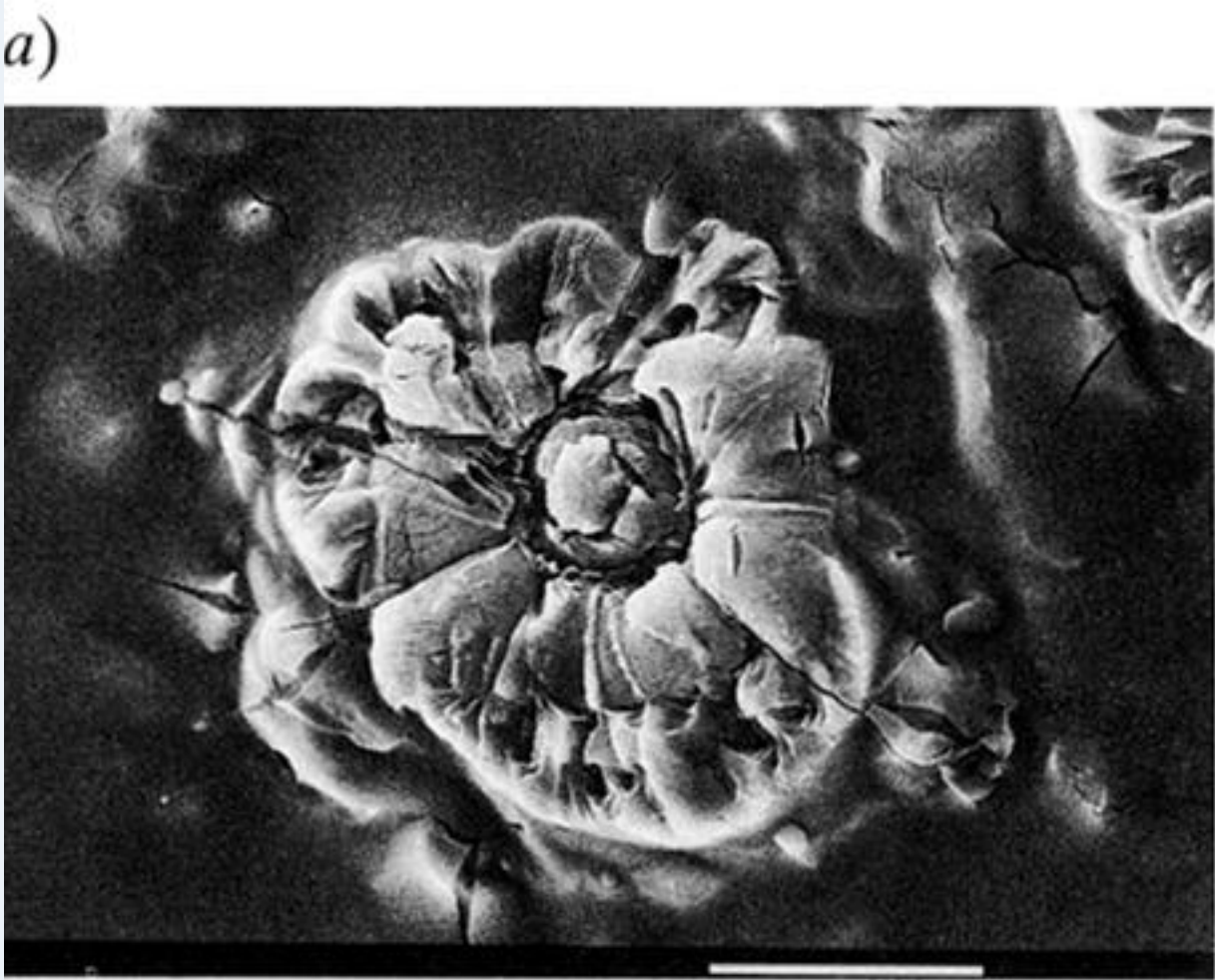
Figure 2. Characteristic surface textural features found on surfaces of partially dehydrated crystals ( \phi = 0.43 at 453 K). These features are identified as sites of collapsed bubbles acting as vent holes for the escape of steam from intracrystalline pores within which the volatilized water is temporarily retained. (Scale bars: both 10 \mu\text{m} .)
